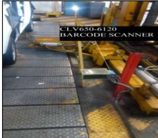
Figure 4.25: Scanner CLV650-6120 in the cage
