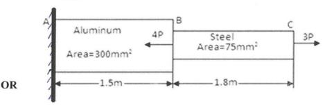
Determine the deflection at nodes and reaction at the support for a spring CO<sub>1</sub> 10 b) assemblage as shown in the figure. Use finite element method
