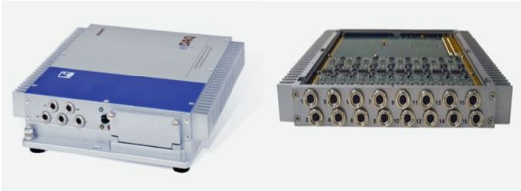
Figure 4.10: e-DAQ Processor and signal conditioning layers
