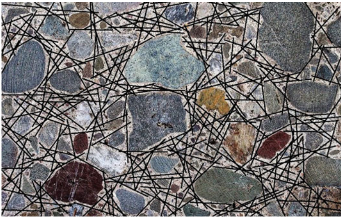
Fig. 1.12 Steel fiber reinforced concrete —The short, discrete fibers (shown by the dark lines ) are randomly dispersed in the concrete at the time of mixing and are present throughout the hydrated cement mortar in the mix. These fiber forms a spatial network around coarse aggregates; wherein, fibers act as ties of imaginary ‘space trusses’ and the mortar mix carries the compression, and also providing anchorage to the fibers. The interfacial transition zone (ITZ) in the concrete, which, otherwise controls the concrete strength properties becomes able to transfer the stresses across the line of discontinuities formed around coarse aggregates by this zone. It also prevents the extension, widening and progress of the microcracks already existing in the ITZ into the adjoining regions in the mortar and their further development in the concrete. The presence of the fibers significantly improves the quasi-brittle characteristics and tensile straining capability of the concrete
