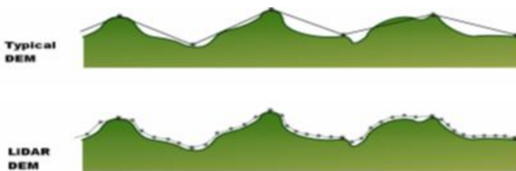
Figure 4.1: Comparative representation of LiDAR survey and Total Station
