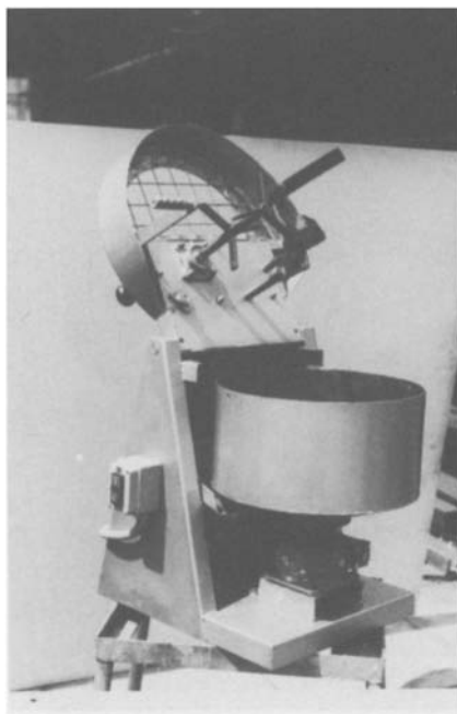
Figure 12.12 Forced action mixer (Edward Benton Ltd)
