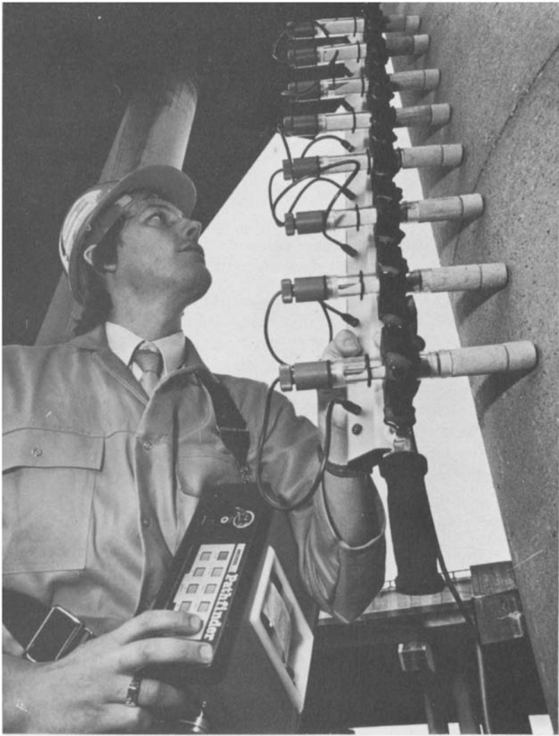
Figure 2.11 Colebrand's Multicell for half-cell potential measurement. The machine reads and records the potentials and displays the values numerically and in graphical format. (Photograph courtesy Colebrand Ltd)
