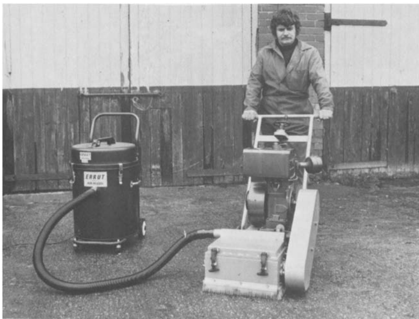
Figure 12.6 Errut planer with vacuum cleaner attachment (British Cement Association)
