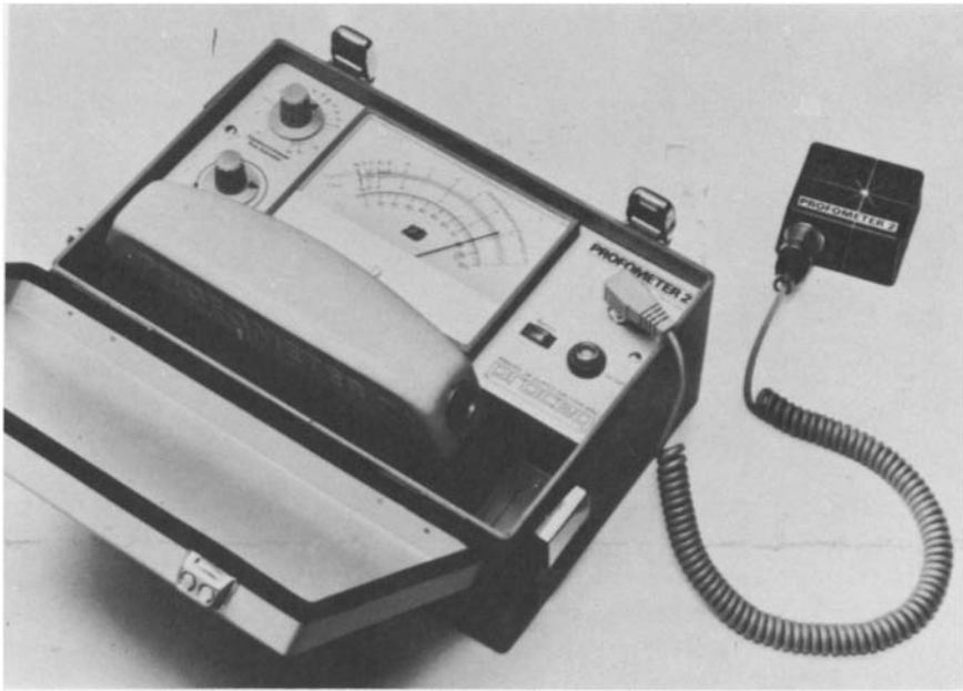
Figure 2.9 Profometer metal reinforcement detector and cover measuring instrument (Proceq SA, Zurich)
