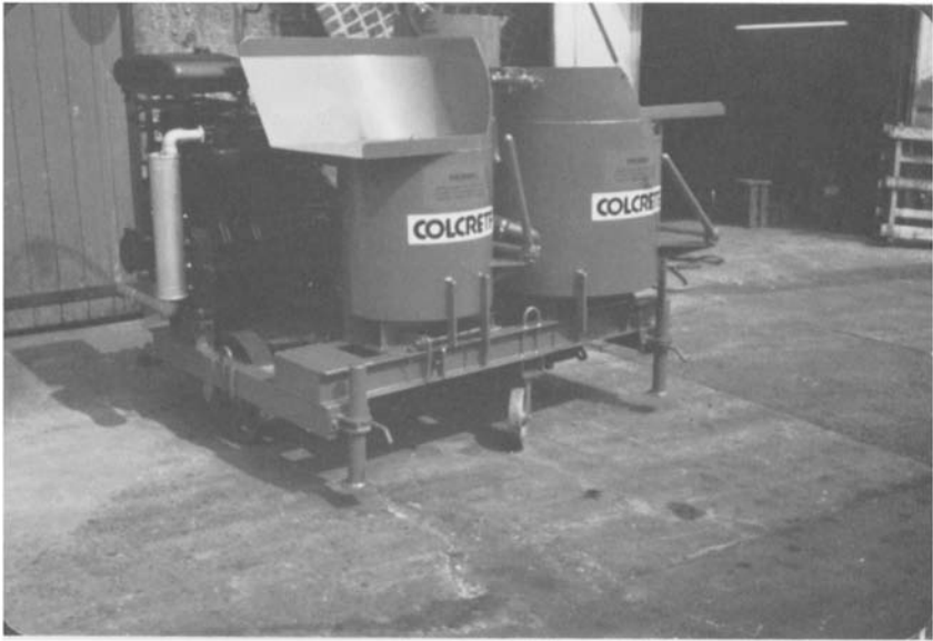
Figure 8.3 High-shear mixer for producing cement grout with reduced tendency for sedimentation (see also Figure 8.4 )
