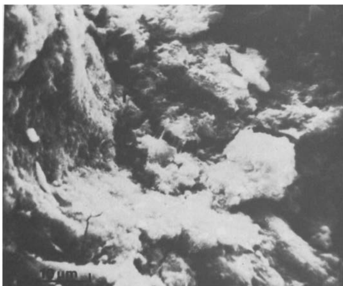
Figure 4.3 Cementitious matrix with SBR latex
