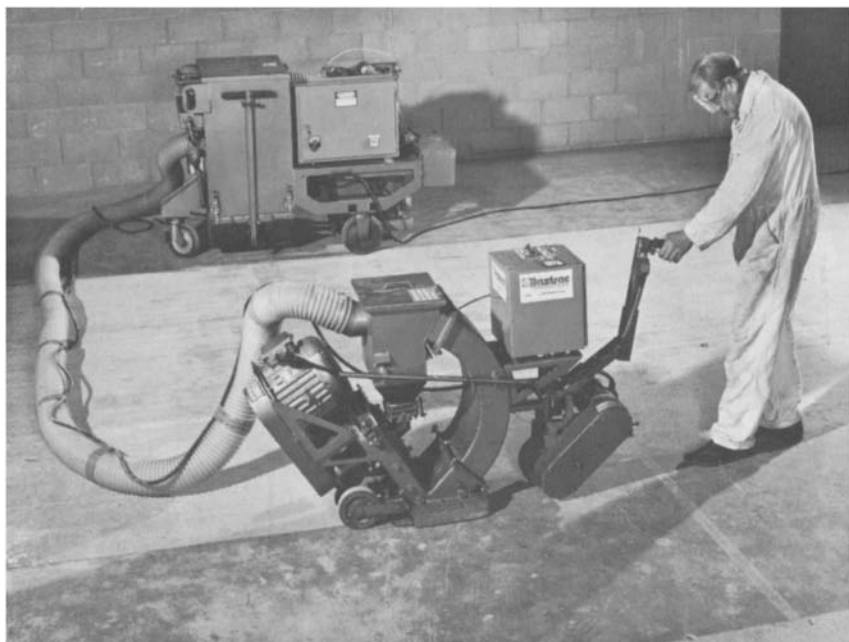
Figure 12.4 The 1–10D Blastrac shot blasting equipment, with a vacuum dust collector unit, on an industrial floor (British Cement Association) affect the depth of surface texture. More than one pass of the machine may be necessary, especially if previous floor finishes such as paint or resin have to be removed (Figure 12.5).
