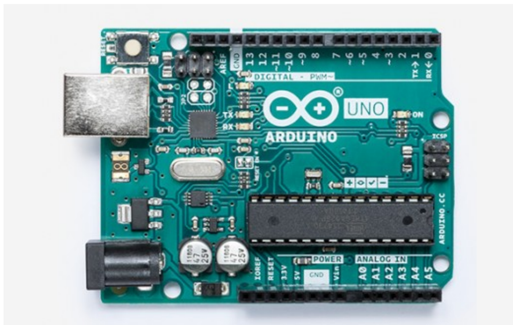
Figure 3.7: Arduino Uno board
