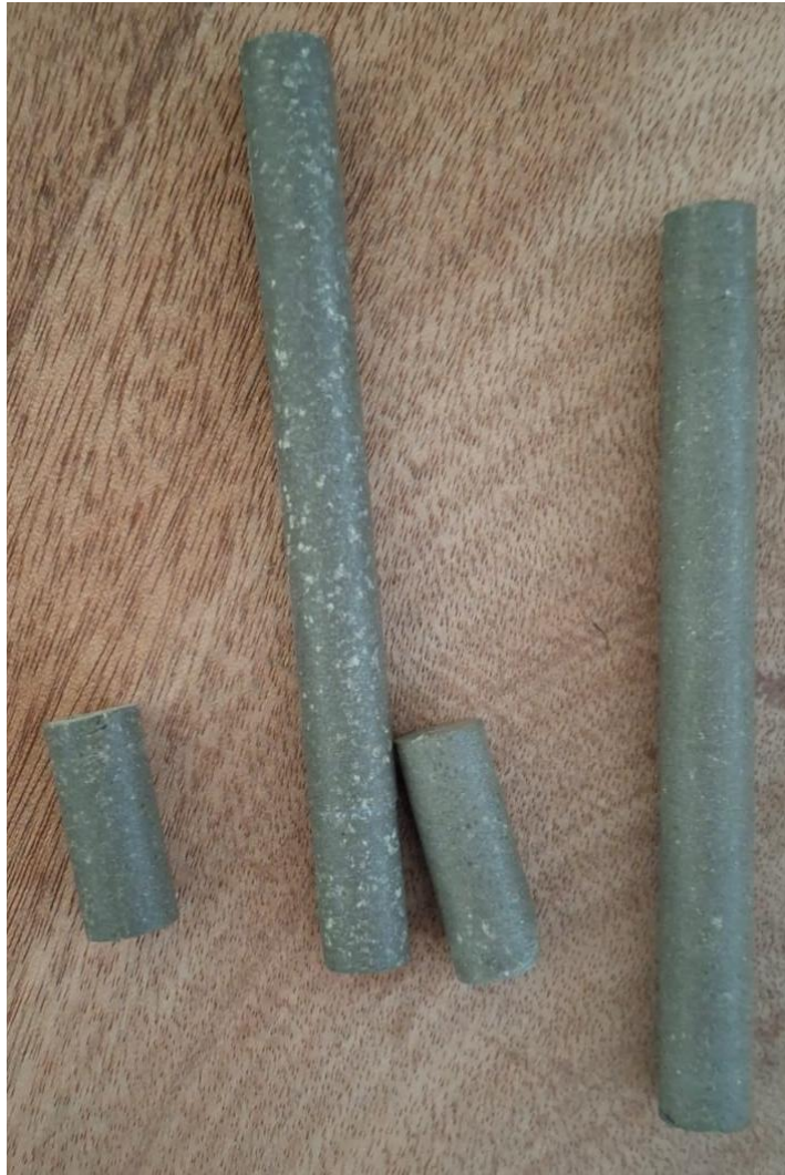
Figure 6.4-Bone pin after removal from Die
