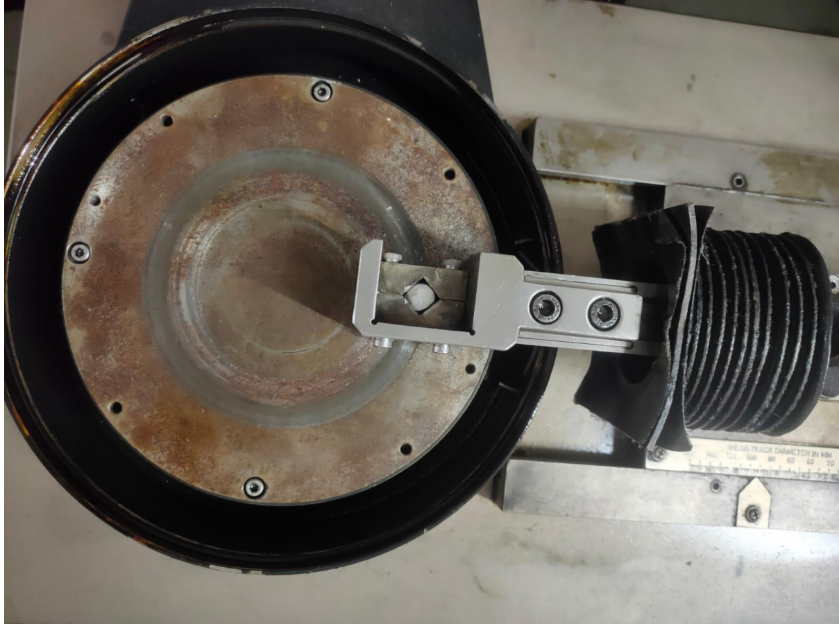
Figure 7.4-Test setup for tribological testing.
