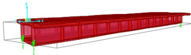
Figure 5.9: Girder Boundary Conditions
