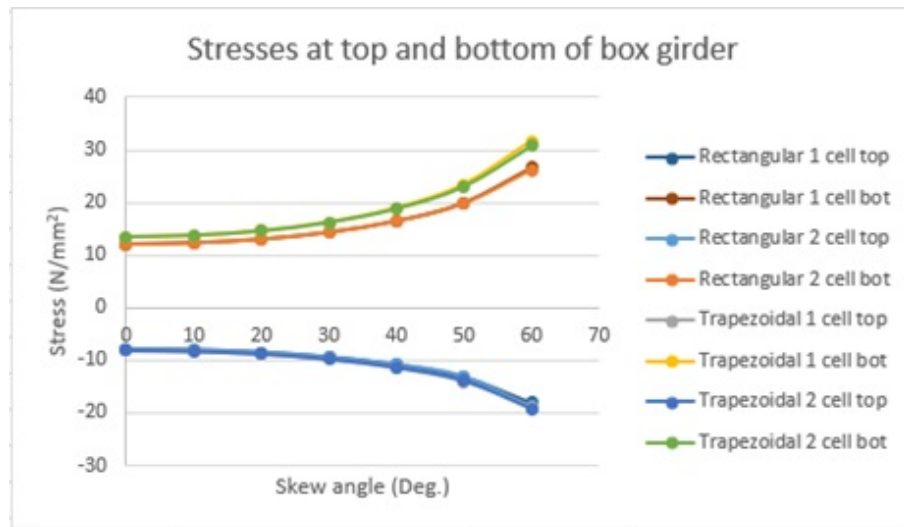
Figure 6.9: Stresses at top and bottom of box girder for increased span N/mm^2
