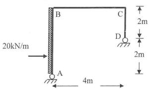
(a) Determine the value of W at collapse load for the portal frame as shown 15 Marks CO1 in figure. All the members have the same plastic moment of resistance.
